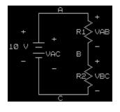
3.a) In the circuit to the left, start at point **C**, and go around the loop in a clockwise (CW) direction. This is loop **CABC**. The KVL equation should be:
