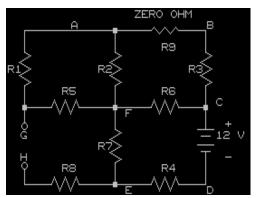
5.a) In the circuit to the left, start at point **A**, and go around the **ABCDEHGA** loop in a clockwise direction.
