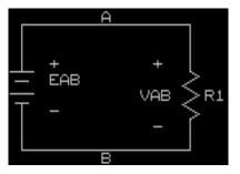
In the diagram to the left,  $E_{AB}$  is the voltage of the voltage source, expressed as "the voltage at node A compared to the voltage at node B." It's actually unnecessary to have the + and - signs shown, since  $E_{AB}$  says it all.
