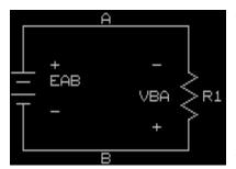
2.c) In the circuit to the left, we will start at point **B**, and go around the loop in a counterclockwise (CCW) direction. Notice that we enter the positive end of each element. The KVL equation, done this way, is:
