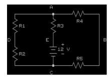
4.a) In the circuit to the left, start at point **D**, and go around the **DAECD** loop in a clockwise direction. Notice that the + and - signs for resistor polarities are not shown - recall that they are not needed. For example the voltage across resistor R1 can be expressed as  $V_{AD}$  (+ at top, - at bottom), or as  $V_{DA}$  (+ at bottom, - at top); either one is fine.
