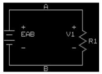
In the diagram to the left,  $E_{AB}$  is the voltage of the voltage source, expressed as "the voltage at node A compared to the voltage at node B." It's actually unnecessary to have the + and - signs shown, since  $E_{AB}$  says it all.
