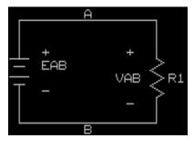
2.d) In the circuit to the left, we will start at point **B**, and go around the loop in a counterclockwise (CCW) direction. Notice that we enter the negative end of the resistor, and the positive end of the battery. The KVL equation, done this way, is:
