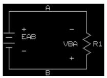
2.a) In the circuit to the left, we will start at point **B**, and go around the loop in a clockwise (CW) direction. Notice that we enter the negative end of each element. The KVL equation, done this way, is:
